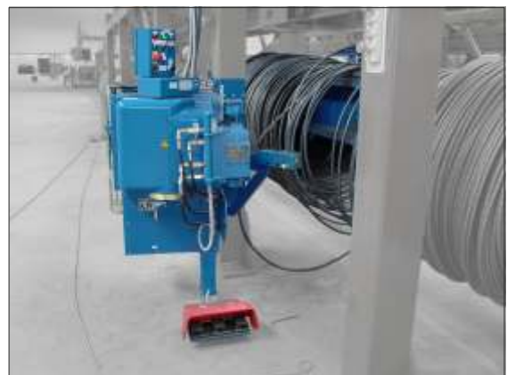
3a-NV with vertical hydraulic clamping device pivoting into the horizontal line
