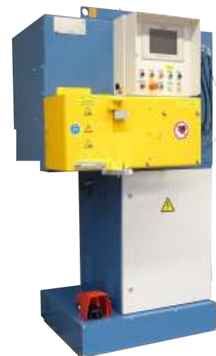
SS 80-FPC with vertical hydraulic clamping device motor driven in one axis or pivoting into the horizontal line
