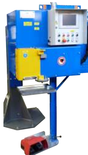
SS 80-FPC with vertical hydraulic clamping device motor driven in one axis or pivoting into the horizontal line
